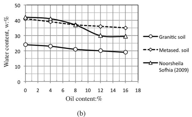
FIGURE 3. Results of the Atterberg limits tests on graniti and metasedimentary soils (a) liquid limit (b) plastic limit
